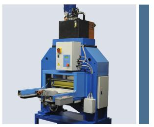
Power 50 tons - 400 V - electric equipment Working area 550x400 mm
