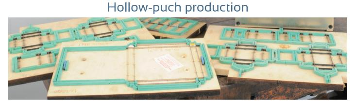
Made of steel or wood (American type) on client's request, for any type of punchable material, with cut and creasing. Our hollow punches can be mobile or fixed directly on the push surface.
