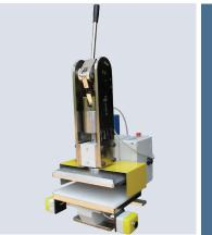
Power 10 tons - 230 V manual or electric equipment Working area 350x250 mm
