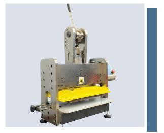
Power 15 tons - 230/400 V - electric equipment Working area 550x400 mm
